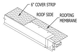
**STEP 5: Installing Approved Roofng Membrane**Install 6" Cover Strip per roofing manufacturer's instructions,
