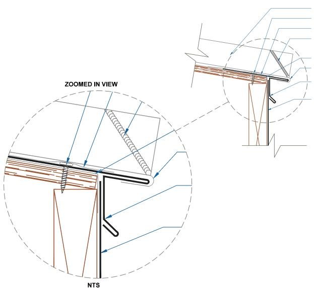
DMC 200S PANEL #10 - 13 x 1" PHW (12" o.c.) METSHIELD UNDERLAYMENT DREXEL APPROVED TUBE SEALANT (FIELD APPLIED BETWEEN PANEL RIBS) METSHIELD UNDERLAYMENT FIELD CUT & HEM PANEL 180°
