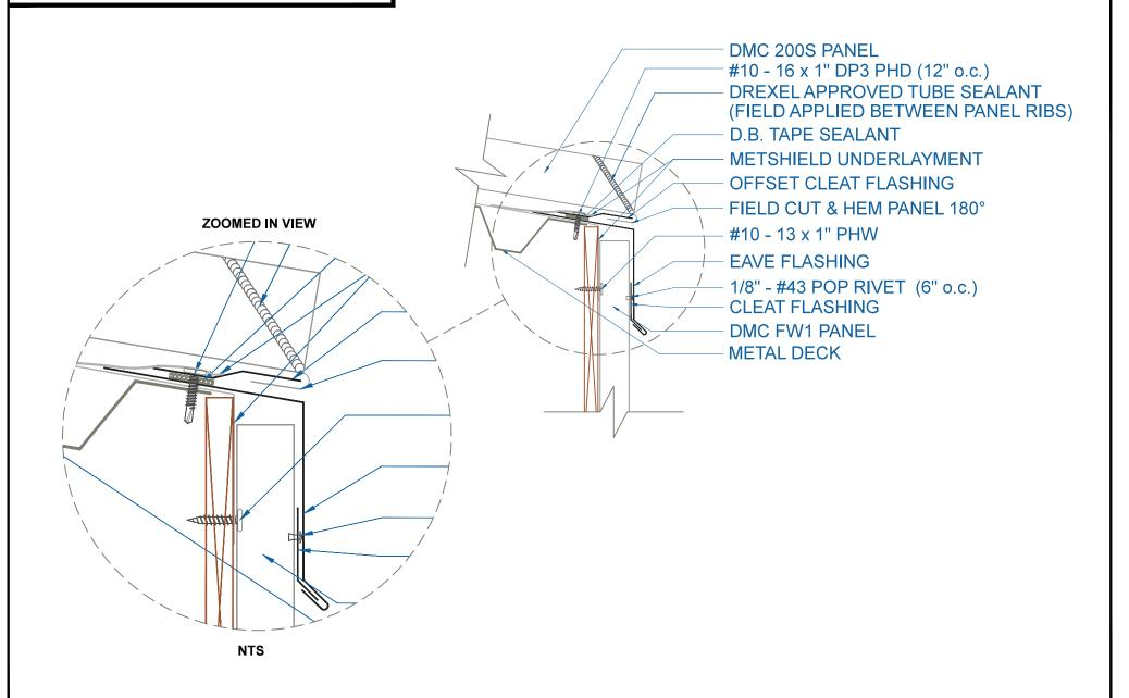
EAVE w/FLUSH PANEL Drexe Metals SCALE: 3" = 1'-0"
