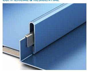
Installation ease with impeccable results makes our DMC 15OSL roof system a standout choice. The 1-1/2" Snap Lock profile and DMC 15OSL Clip create a continuous interlocking system that installs quickly, reducing labor costs. The concealed fastener and clip application also allow thermal expansion and contraction movement to help keep the beautiful finish straight and true.
